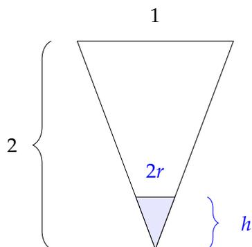
The side view of the tank forms a triangle that is similar to the triangle formed by the side view of the water, so
