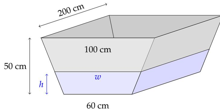
We can calculate the volume of water in the trough by multiplying the area of its trapezoidal cross section by 200 cm. A trapezoid with height  $h$  and bases  $b_1$  and  $b_2$  has area  $h \left( \frac{b_1 + b_2}{2} \right)$ . (To see why this is so, draw the trapezoid as a rectangle flanked by two triangles.) So, using  $w$  as the width of the top of the water (as in the diagram above), the area of the cross section of the water in the trough is
