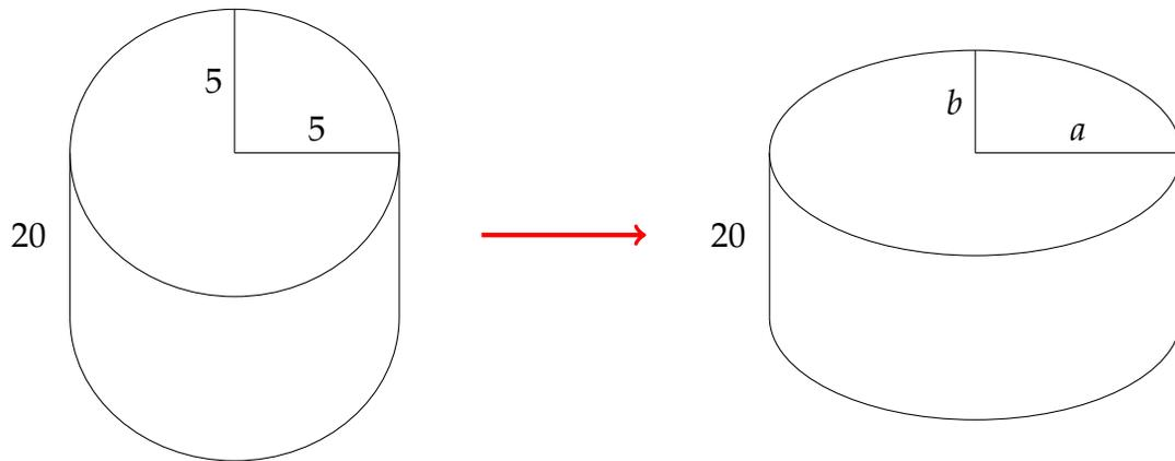
After  $t$  seconds of smooshing the bottle,  $a = 5 + t$  cm. The perimeter of the cross section is unchanged as the bottle deforms. The perimeter of an ellipse is actually quite difficult to calculate, but we will use an approximation derived by Ramanujan and assume that the perimeter  $p$  of our ellipse is
