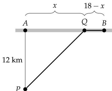
Using the Pythagorean Theorem, the distance from  $P$  to  $Q$  is  $\sqrt{12^2 + x^2}$  kilometres, and the buggy travels 15 kph over this off-road stretch. The travel time from  $P$  to  $Q$  is  $\frac{\sqrt{12^2 + x^2}}{15}$  hours.
