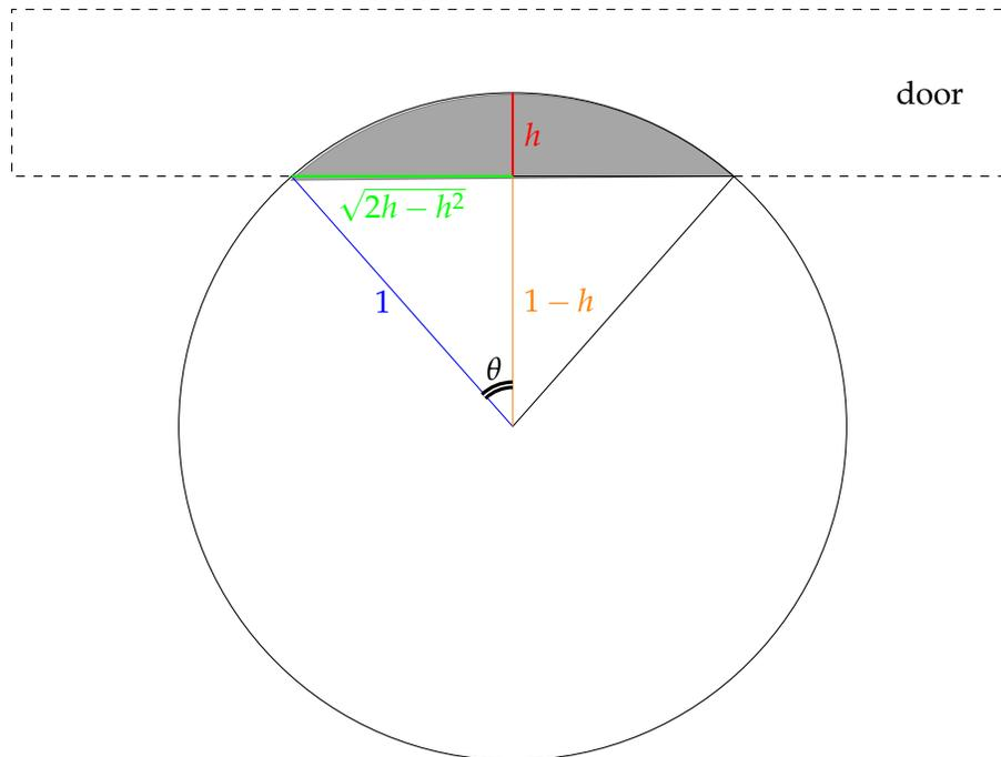
Since the radius of the pipe is 1 metre, the orange line has length  $1 - h$  metres, and the blue line has length 1 metre. Using the Pythagorean Theorem, the green line has length  $\sqrt{1^2 - (1 - h)^2} = \sqrt{2h - h^2}$  metres.
