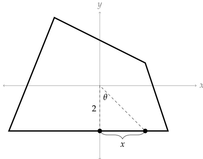
When the point is a little to the right of  $(0, -2)$ , then we can make a triangle with the origin, as shown. If we let  $\theta$  be the indicated angle, then  $\frac{d\theta}{dt} = 1$  radian per second. (It is given that the observer is turning one radian per second, so this is how fast  $\theta$  is increasing.) From the right triangle in the diagram, we see
